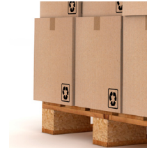
Pallet overhang 50% loss in strength
