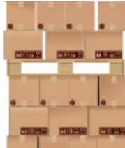
Pallet deck misalignment 32% loss in strength
