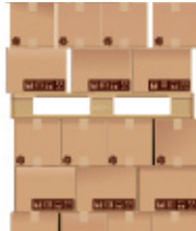
Pallet deck misalignment 32% loss in strength
