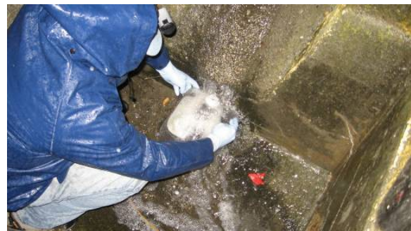
Figure 9. Collecting a sheet flow stormwater sample.
